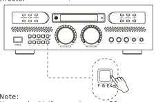
Use mode #1 if room size over 30 square meters. Use mode #2 if room size between 20~30 square meters. Use mode #3 if room size below 20 square meters.
